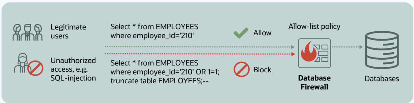
Figure 8.2: Monitoring SQL network traffic with Oracle Database Firewall
